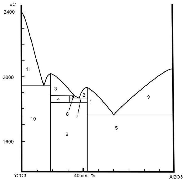
**Figure 1: System state chart Al<sub>2</sub>O<sub>3</sub>-Y<sub>2</sub>O<sub>3</sub>:**
