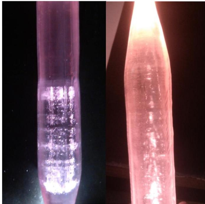
**Figure 2: The perovskite inclusions number increase in the bottom of the crystal.**
